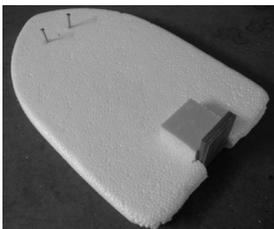
Screw and Anchors Installed Near Front of Board Spaced For Battery
